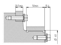
Assembly accessories: Mounting kit consisting of stainless steel screws, discs, seals and O-rings.
