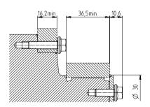
Assembly accessories: Mounting kit consisting of stainless steel screws, discs, seals and O-rings.
