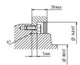
Non-tolerated dimensions are nominal dimensions  $^{\prime\prime}$  Check motor shaft fit  $^{\prime\prime}$  Min./Max. permissible motor shaft length. Longer
